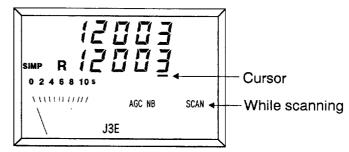
3. To stop scanning, press the **SCAN** key or the **PTT** switch. "SCAN" disappears from the LCD.
